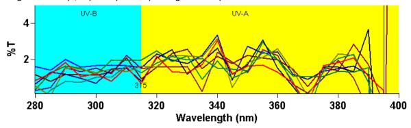
Following the determination of the sun protection factor, it was found that both developed prototypes exhibit excellent levels of sun protection (SPF > 50+), with measurements conducted in the 400–280 nm range. Specifically, knit 1 shows an SPF of over 58, while knit 2 has an SPF of over 67.
